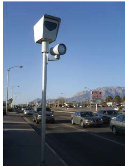
This camera system identifies violations of red-light signals at an intersection, transmitting evidence and vehicle identification information to the vendor. Vendors issue tickets, after approval by local authorities, which are then delivered to the registered owner of the vehicle. Credit: Flickr user Busboy4, Creative Commons
