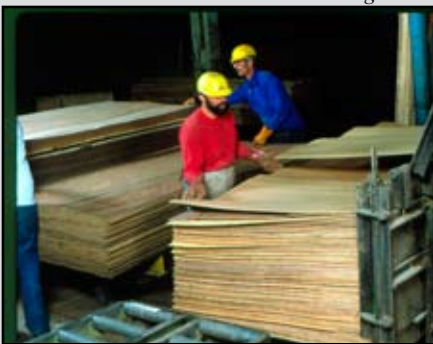
Workers stack sheets of Columbia Forest Products' hardwood plywood, a product made with an innovative formaldehyde-free adhesive called PureBond.
