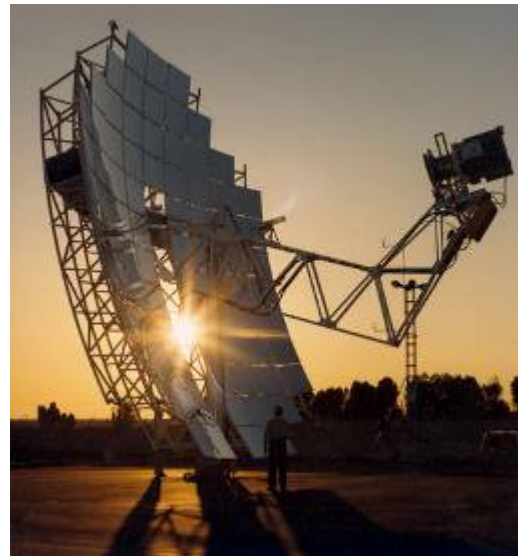
Concentrating solar power technologies, like this dish-engine system, have made great advances thanks to federal research and development efforts. Credit: DOE/NREL, Stirling Energy Systems.
