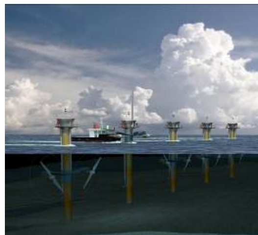
Turbines like the ones in the diagram above could be used to harness the power of tidal energy. Credit: Marine Current Turbines.
