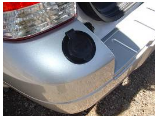
The socket on the bumper of this plug-in hybrid electric vehicle allows the user to recharge the vehicle’s battery using power from the electric grid, reducing the need for gasoline. Credit: DOE/NREL, Keith Wipke.
