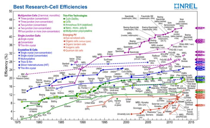
This chart from the National Renewable Energy Laboratory illustrates the steadily improving efficiency of solar photovoltaic systems in converting sunlight to energy – as well as the emergence of a variety of new photovoltaic technologies with the potential for breakthrough performance in the years to come.
