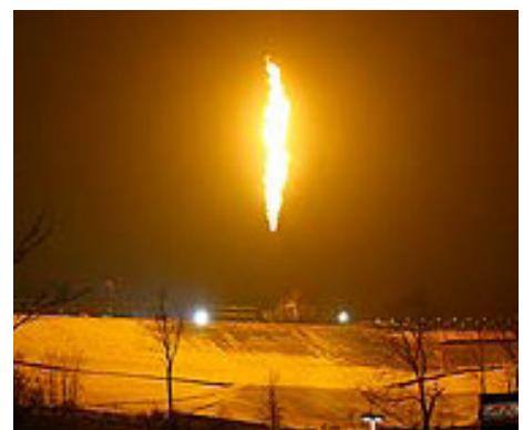
Flaring or burnoffs often burn unevenly due to wind and other atmospheric variables resulting in methane and other gases being released into the air.
