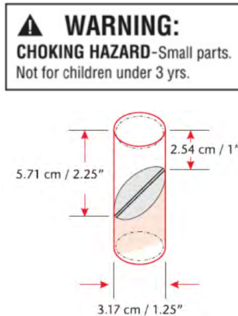
Figure 1. Choke Test Cylinder
