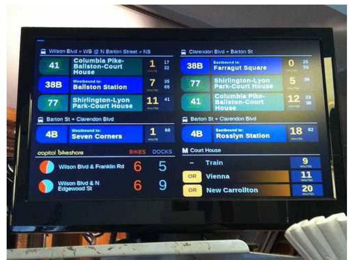
Informational screens, such as this TransitScreen in Washington, D.C., provide up-to-the-minute data on the location of buses and availability of bikeshare docks.
