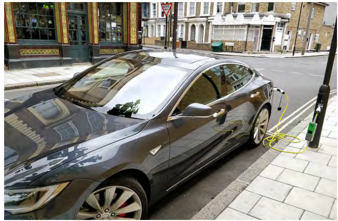
Electric vehicle charging port on a lamppost. Photo: Jason Cartwright via Flickr, CC BY 2.0.
