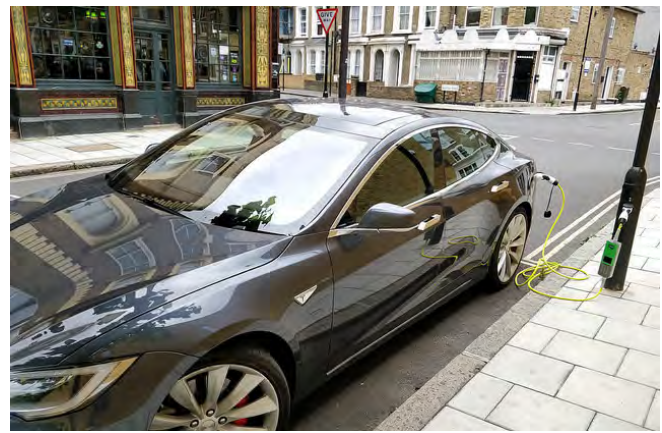
Electric vehicle charging port on a lamppost. Photo: Jason Cartwright via Flickr, CC BY 2.0.
