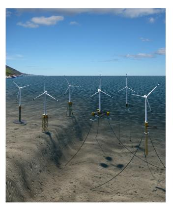
This National Renewable Energy Laboratory diagram displays various designs for offshore wind turbines, including commonly-used monopiles on the far left, and floating designs on the right. Modern monopile technology allows for affordable installations in waters up to 40 meters deep, while floating turbines dramatically expand the ocean areas feasible for offshore wind. Image: NREL.
