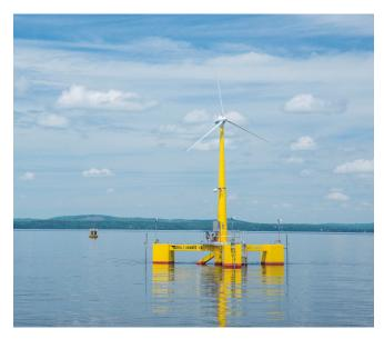
University of Maine researchers are developing new floating wind turbine technology. This turbine above is a 1:8 scale prototype used for testing off the coast of Castine, Maine. The project is planning to eventually deploy two full-size 6 MW turbines. Image: Courtesy of University of Maine
