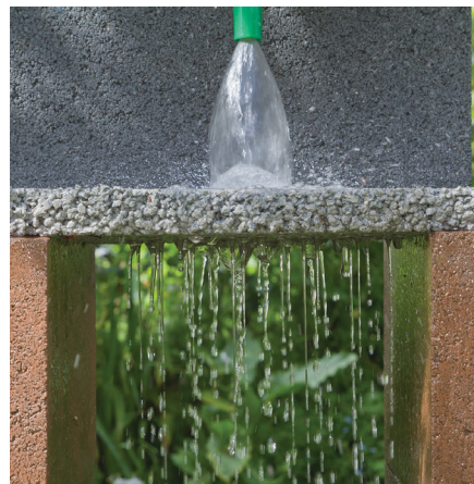
▲ Permeable pavement that allows water to soak through is an example of Green Stormwater Infrastructure that could help mitigate flooding.
