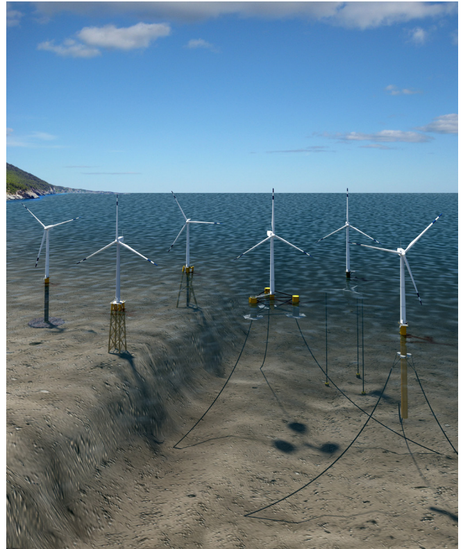
This National Renewable Energy Laboratory diagram displays various designs for offshore wind turbines, including commonly-used monopiles on the far left, and floating designs on the right. Modern monopile technology allows for affordable installations in waters up to 40 meters deep, while floating turbines dramatically expand the ocean areas feasible for offshore wind. Image: NREL.
