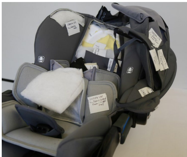
Children's car seat with samples of fabrics, foam, and plastic removed and labeled.
