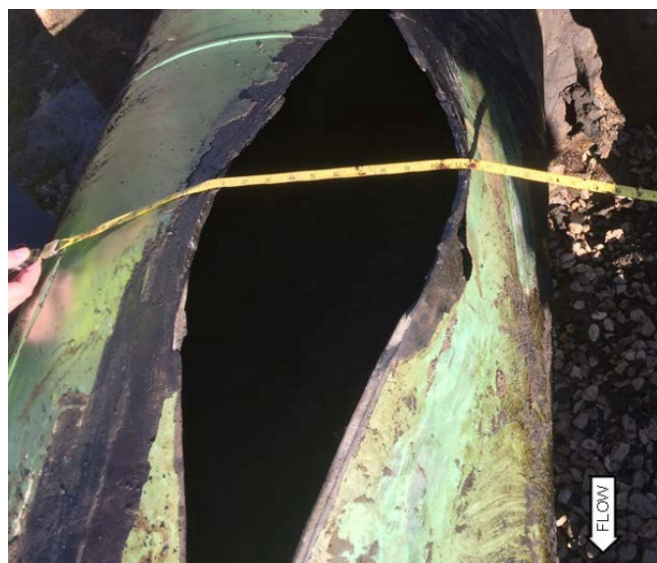
This rupture in the Keystone Pipeline near Amherst, South Dakota, led to the spill of approximately 5,000 barrels of oil. 113 Image: National Transportation Safety Board
