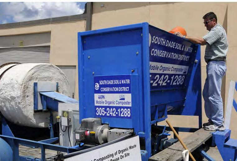
*Feeding an in-vessel composting machine on Homestead Air Reserve Base.* Credit: Lou Burton via U.S. Air Force, CC-BY 1.0.
