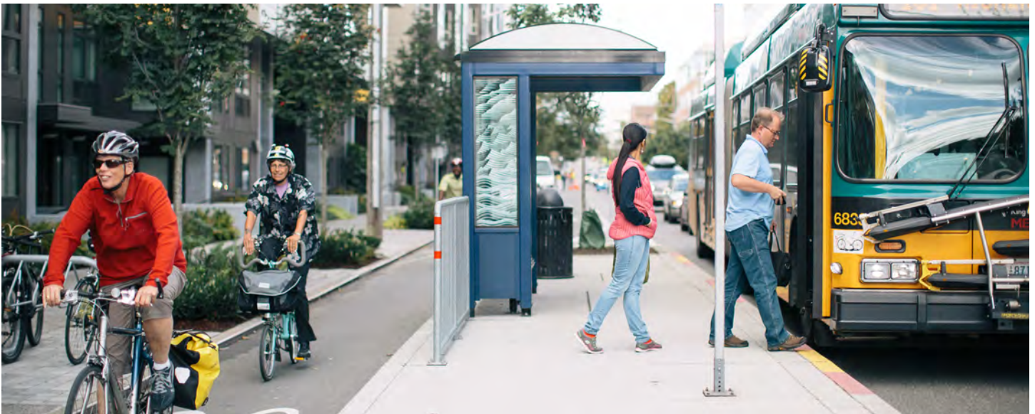
By designing streets to serve pedestrians, bicyclists and transit – including by adding infrastructure like this bike lane and floating bus stop in Seattle – cities can encourage low-carbon transportation and make streets safer for everyone. Credit: Adam Coppola Photography via Flickr (public domain)
