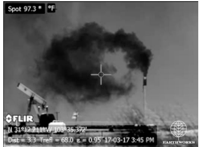
The image on the right shows methane spewing from an unlit flare, which is invisible to the naked eye, in Reeves County.
