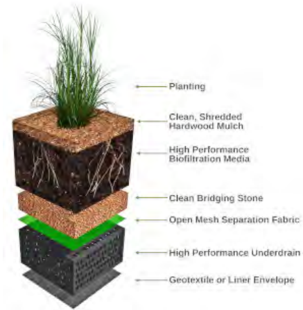
Focal Point biofiltration system. Credit: Convergent Water Tech
