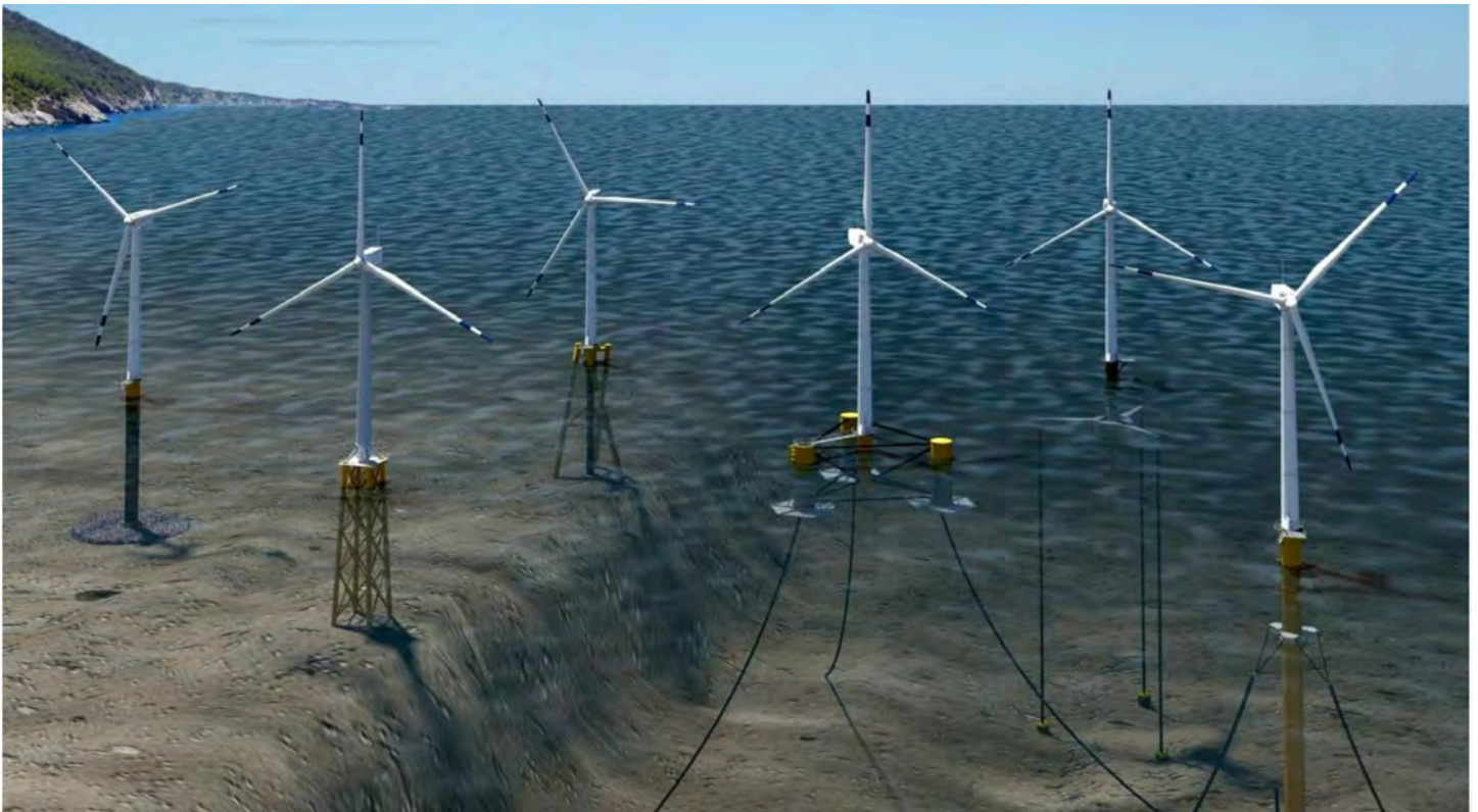
From left to right: a monopile, jacket, twisted tripod, floating semi-submersible, floating tension leg platform and floating spar. Image: Josh Bauer/NREL-Department of Energy 41
