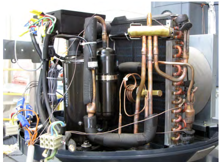
Heat pump components in an integrated heat pump water heater. Photo credit: Kate Hudon / NREL
