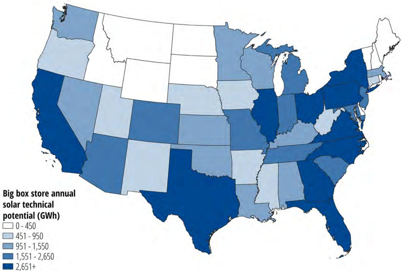
Figure ES-1. Big box store solar PV technical generation potential, by state
