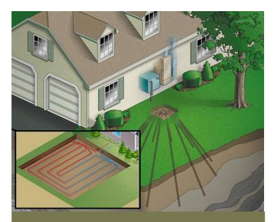
Ground source heat pumps use the earth as a heat source in the winter or as a heat sink in the summer, benefiting from the earth's stable temperature.
