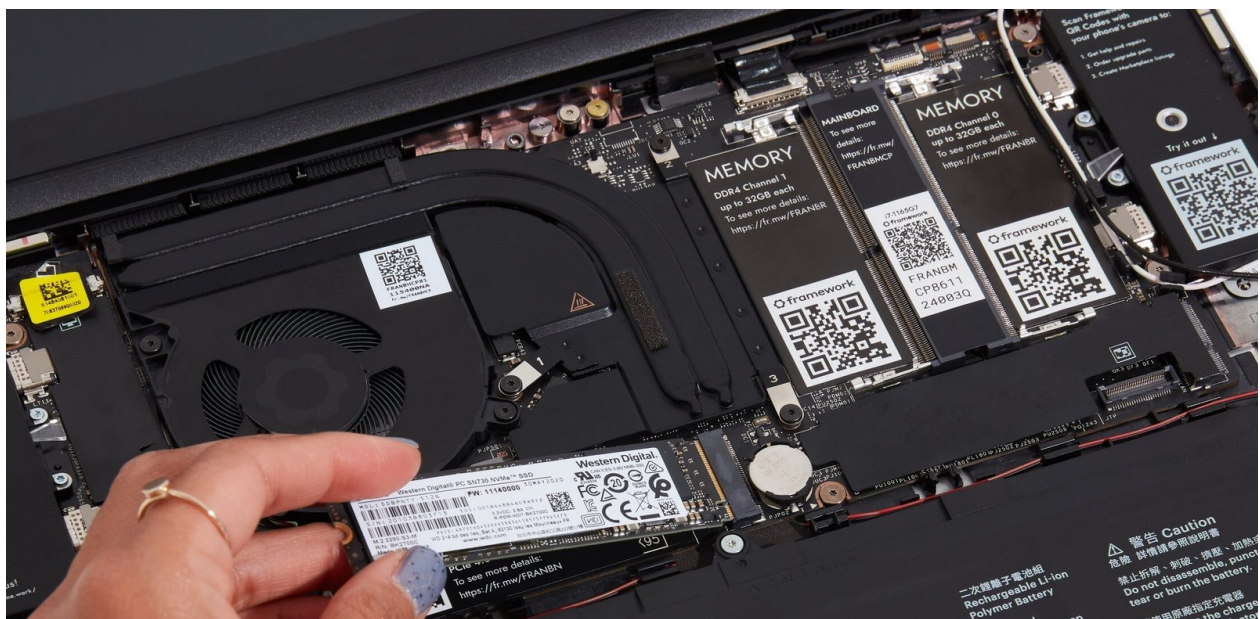
Figure 11: Framework's on-component QR codes enable easy repair access.
