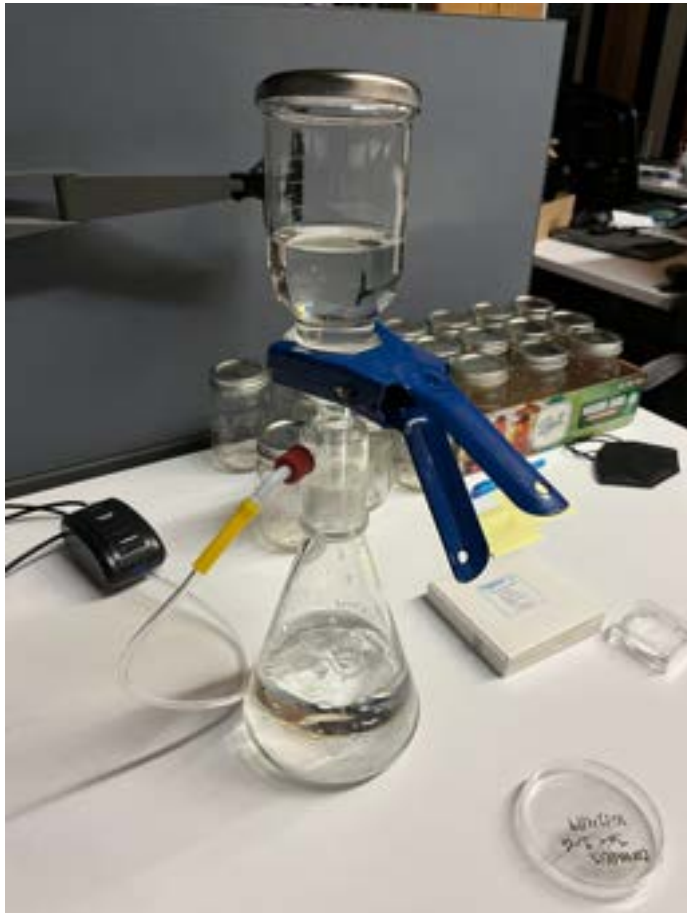
A water filter funnel with a motorized pump processes a sample.
