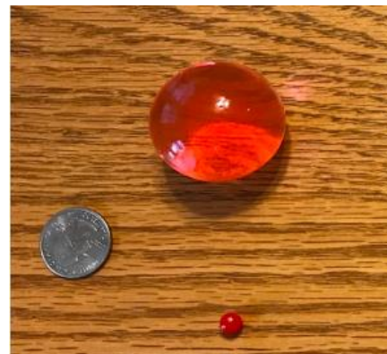
This photo shows a water bead at original size, and then how it expands after combined with water. We show a quarter for scale.
